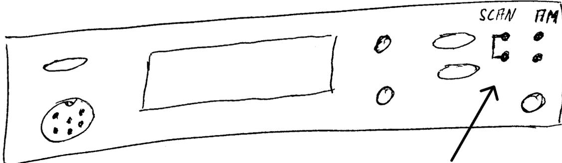
Please open this jumper and solder a new jumper into the holes named "AM"
