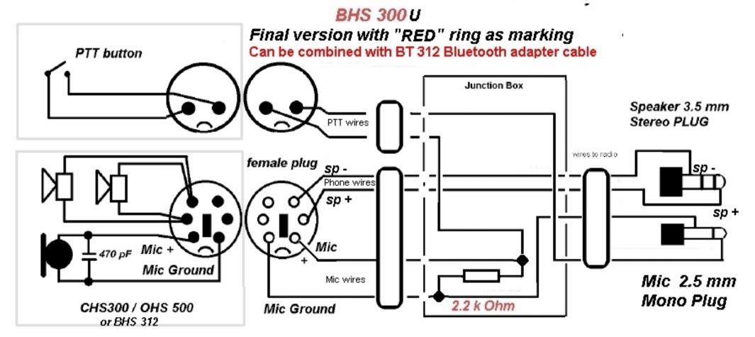
Difference to "reworked" and "blue"marked BHS 300 U: PTT switch is in series with MIC + and reversed speaker connection at 3.5 mm socket
